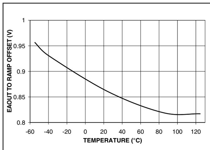
Figure 6. EAOUT to RAMP offset over temperature.
