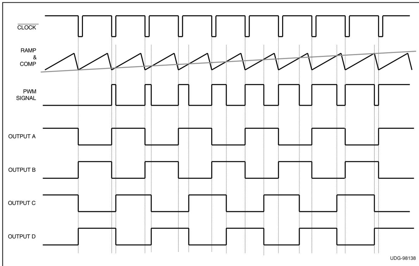
Figure 4. UCC3895 timing diagram (no output delay shown).
